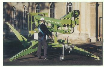
Fully proportional hydraulic outriggers make setting up and levelling quick and easy even on gradients.
